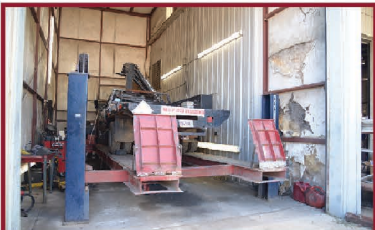
Hunter Truck Lift TR25PL-25,000 pd capacity
